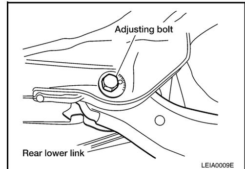
8. Tighten the adjusting bolt nuts to the specified torque.
