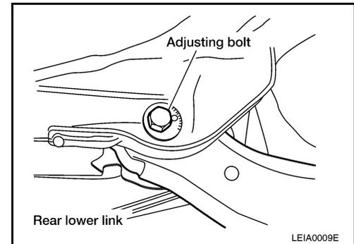
2. Tighten the adjusting bolt nuts to the specified torque.
