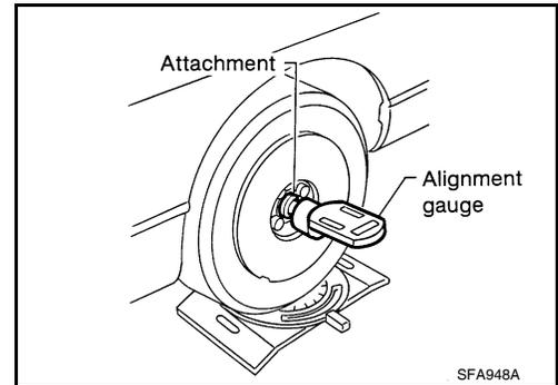
1. Turn the adjusting bolts in the same direction to calibrate.
